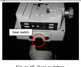
Figure 19. Gear switches
